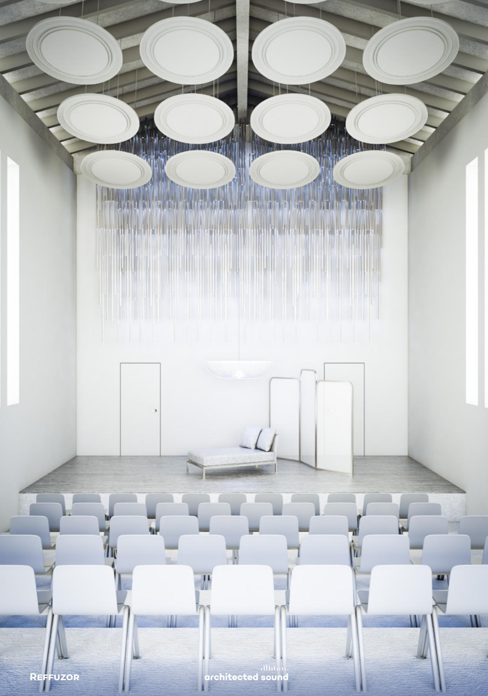
Reflective panels over the stage can be used as an alternative to full ceilings with sculpted geometry. Unlike standard ceiling solutions, REFFUZOR panels do not reduce the room volume. Additionally, due to the possibility of differentiating possible shapes, they will not change the design concept.
